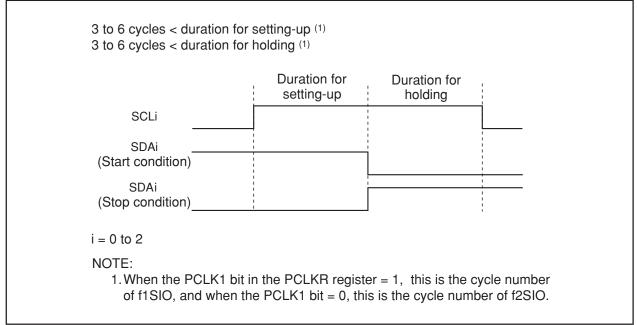
Figure 14.25 Detection of Start and Stop Condition
